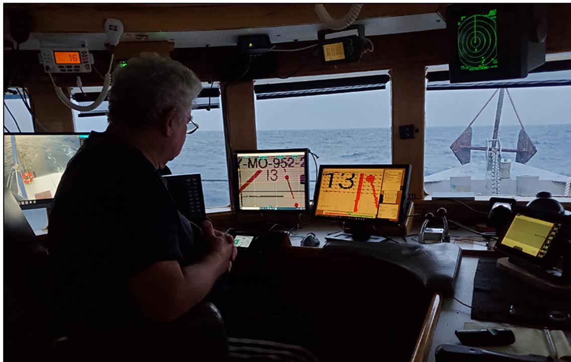
Figure 3-16. Captain Perry Zirlott at the helm of the RV Kimberly Dawn viewing the navigation computer screen. The survey vessel was steered along pre-planned survey track lines by autopilot.
