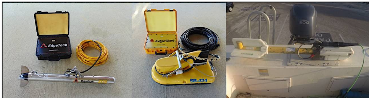
Figure 3-09. Survey instruments employed during the investigation included (from left to right) the sidescan EdgeTech 4125 sonar, the EdgeTech 424 subbottom profiler, and the Geometrics 882 magnetometer.
