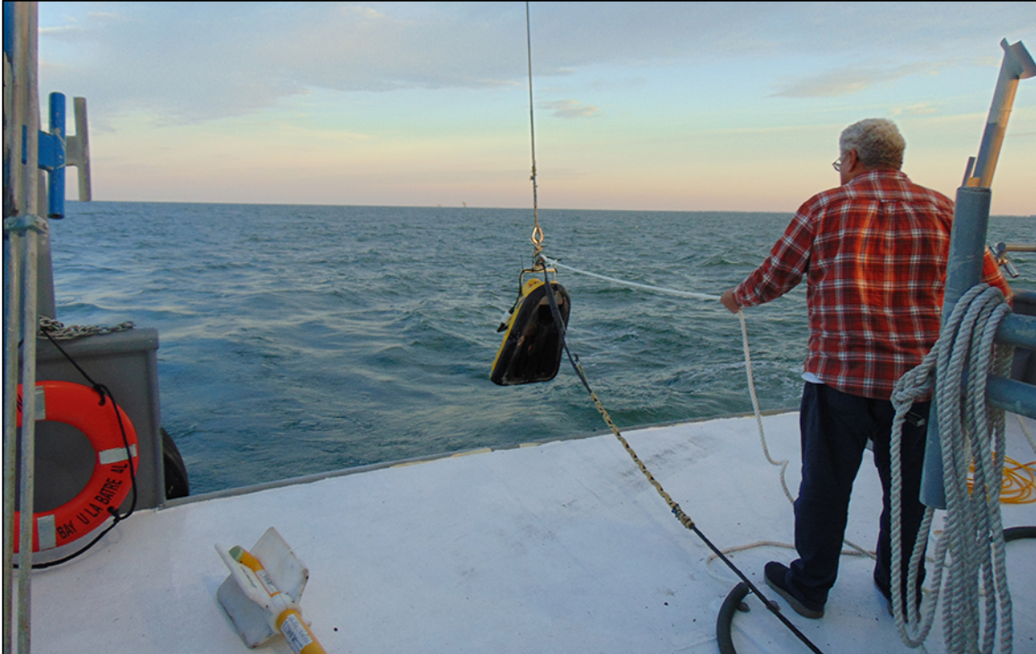
Figure 3-04. General conditions during survey of an offshore cell. Captain Perry Zirlott shown deploying the subbottom profiler. Magnetometer is on the deck at left.
