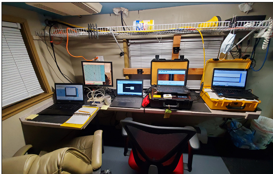
Figure 3-17. Survey computer station. From left to right, two positioning and vessel track computers, magnetometer data computer (center), the sonar data computer, and at right the subbottom data computer.
