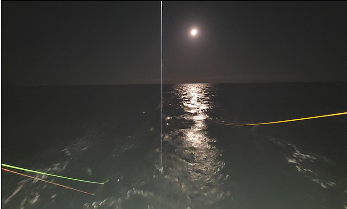
Figure 3-05. Survey at night showing a calm sea. Tethered to vessel's aft A-frame, deployed remote-sensing devices include sonar cable at right, subbottom in center, and magnetometer cable is at left with line for the cable weight to sink the sensor to depth.
