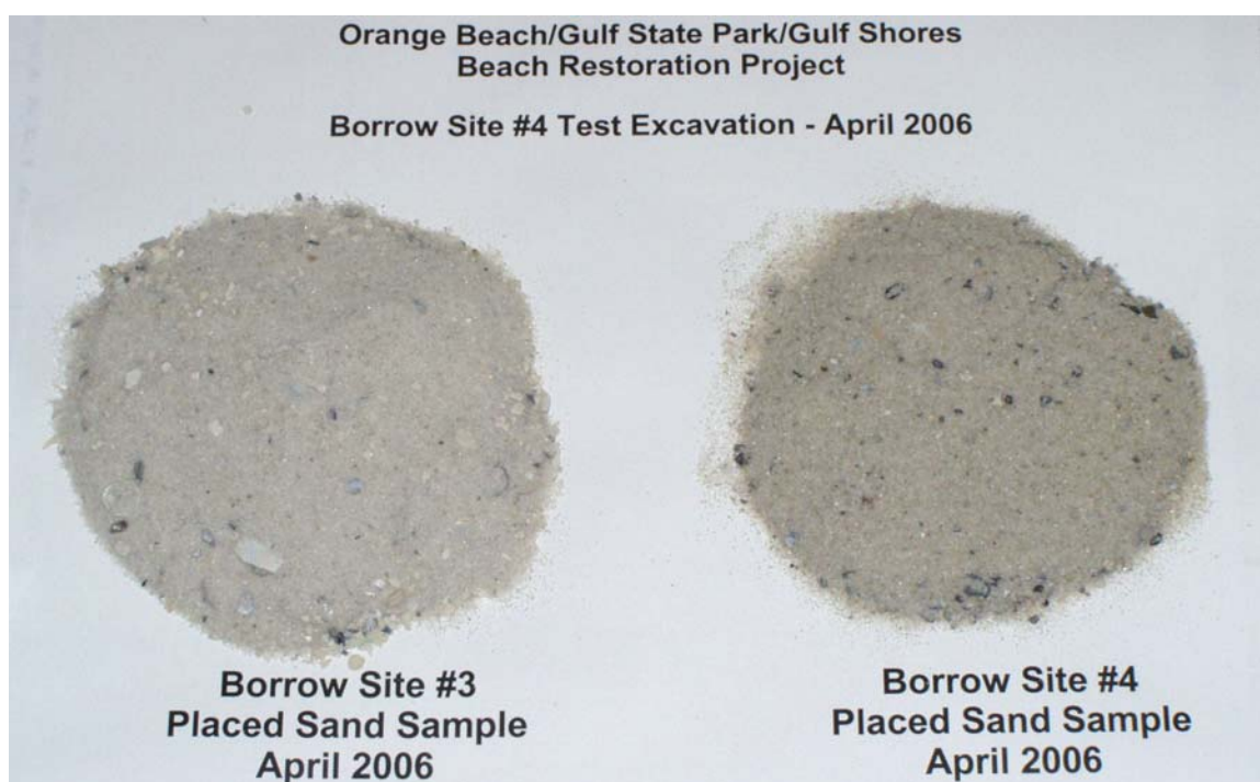
Figure 4.11 Comparison of sediments excavated from Borrow Site #3 off the eastern end of Gulf Shores and Borrow Site #4 located atop Baldwin Shoal, west of Gulf Shores. Color differences depicted in the photo should be considered relative only (for instance - the background for the photo is a nearly-white sheet of paper).
