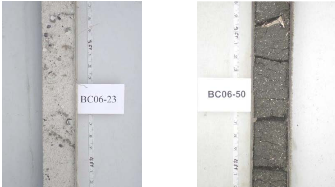
Figure 4.13 Comparison of Vibracore segments collected in the vicinity of Resource Area #1 (Hummell, 1999). These segments, three to four ft below the seabed, lie roughly 1,500 ft apart. Vibracore BC06-23 lies very near Vibracore SR-40 (Hummell, 1999). The segment on the left is classified as white fine quartz sand (10YR 8.5/1) with traces of shell fragments, while the segment on the right is classified as dark gray clay (10YR 4.5/1) with scattered shell fragments and whole shells.
