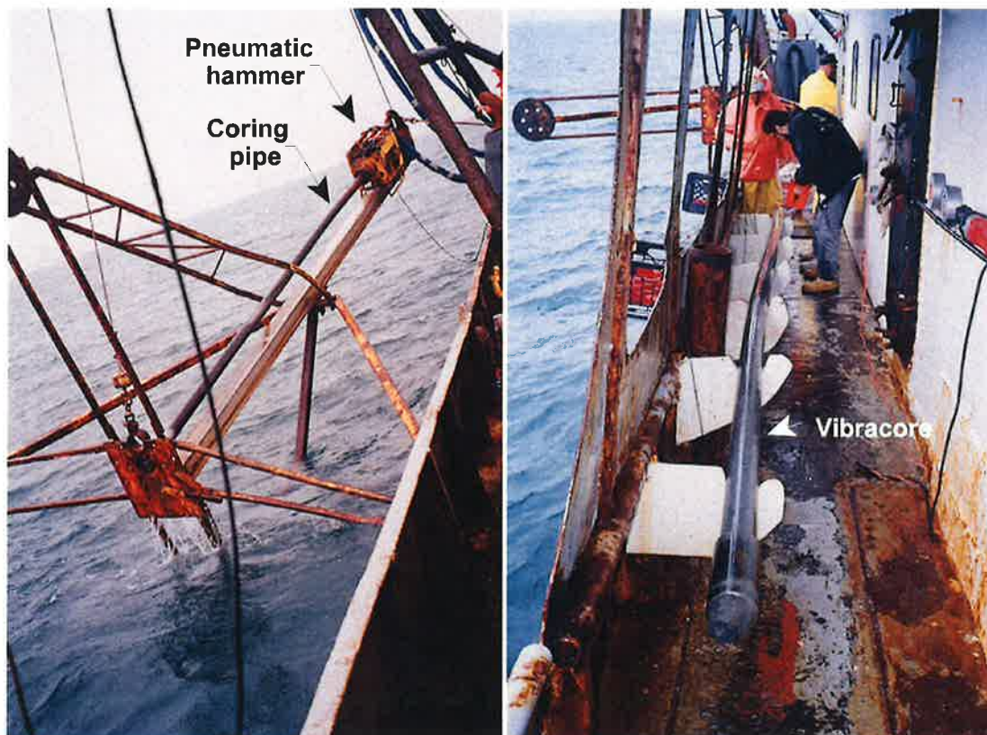
Figure 4.1 Pneumatic core boring rig (left) on the Research Vessel Atlantic Twin, owned and operated by Alpine Ocean Seismic Survey, Inc., of Norwood, NJ. Twenty-foot sediment core ready for labeling and cutting (right).
