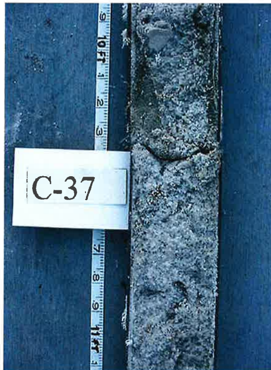
Figure 4.2 Segment of Vibracore Core C-37 collected in the borrow site. The figure shows the white sands in the split core between 10 and 11 feet below the seabed.
