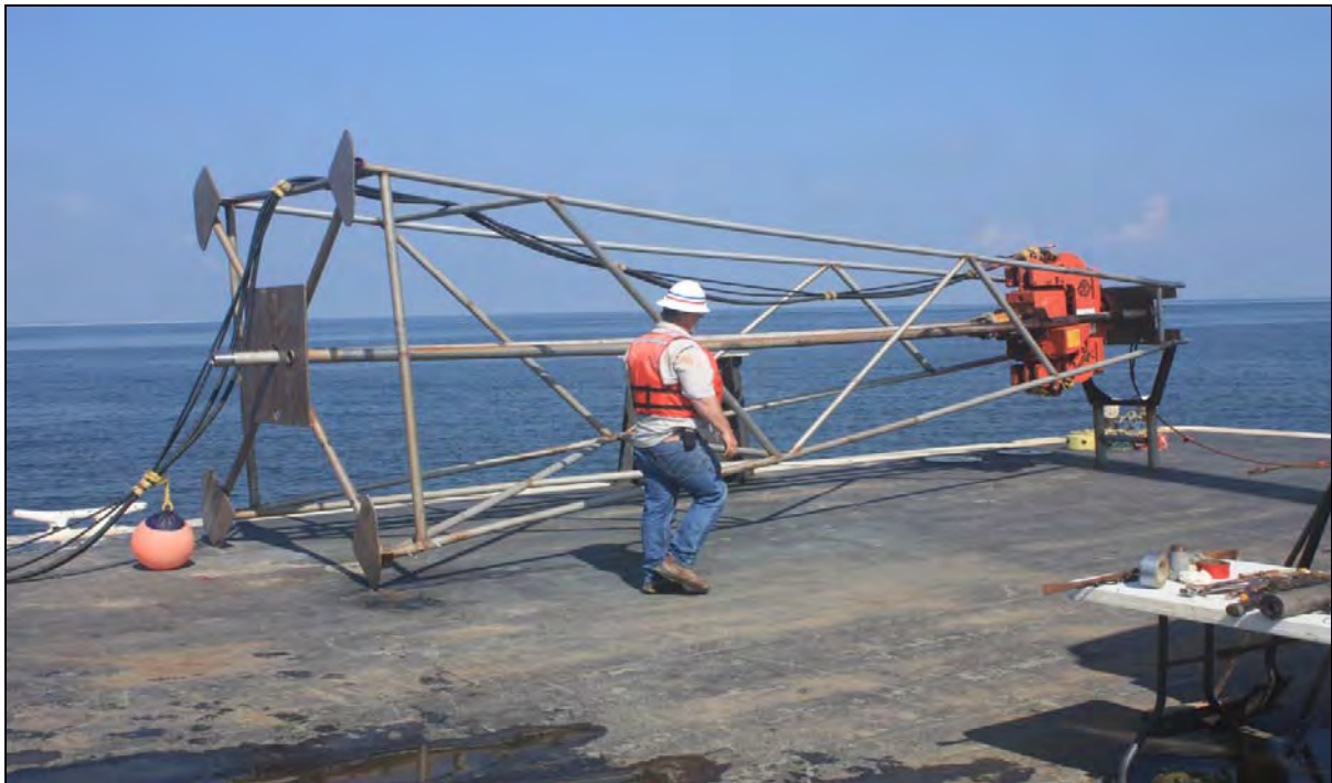
Figure 5.1.1 Vibracore unit used for 2010, 2011, and 2013 sampling events.
