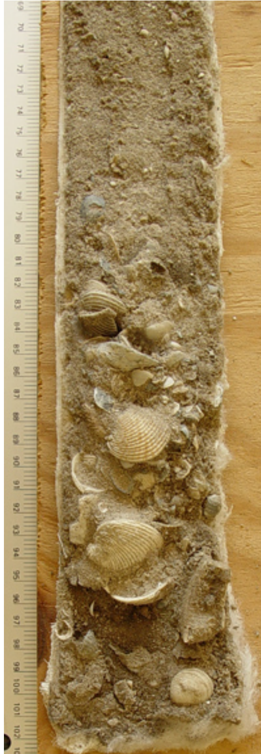
Figure 20. Photograph of peel of coarse shelly lag, Graded Shelly Sand lithofacies, vibracore SR-35, 345-369 cm downcore. Add 267 cm to scale to get true core depth. Interval 69-78 cm is typical of the upper portions of graded units that make up this lithofacies.
