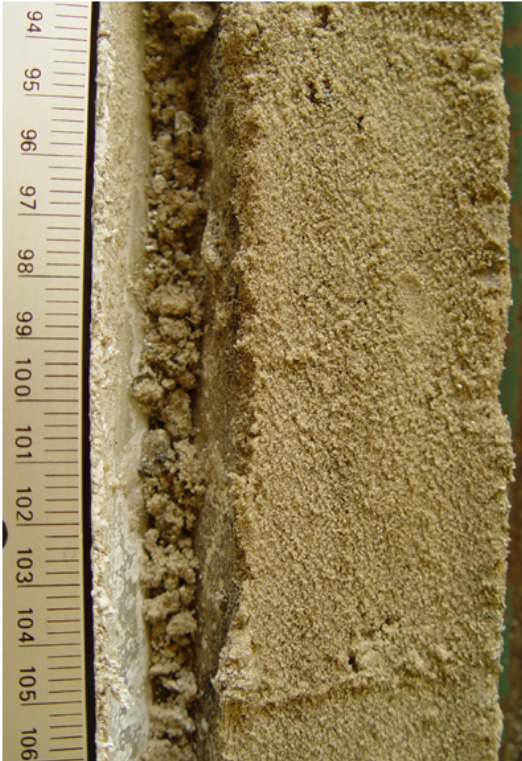
Figure 21. Photograph of Shelly Sand, vibracore SR-100A 93-106 cm downcore. Depth downcore is indicated in centimeters.
