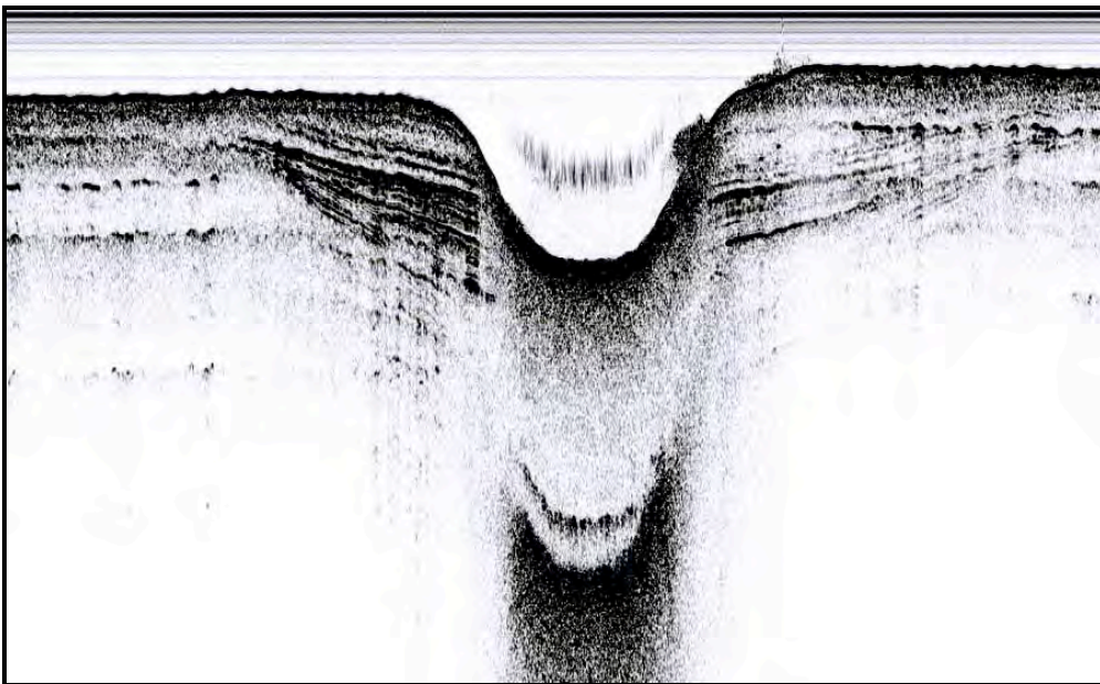
Figure 25. Sub-bottom profile of a sink hole off Cape Romano, Collier County, Florida (Courtesy Coastal Planning and Engineering, Boca Raton, Florida).
