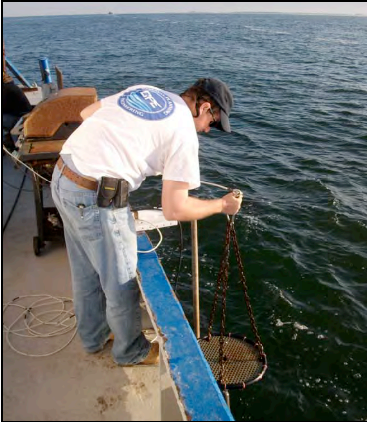
Figure 18. Preparing the bar check disk for deployment.
