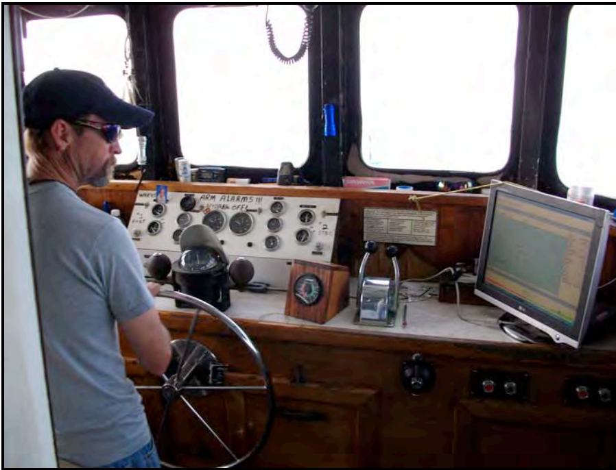
Figure 13. Computer navigation system located at the research vessel helm.
