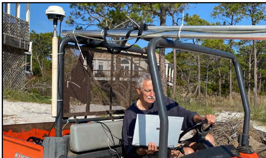
Figure 6. Navigation and data collection were controlled by laptop.
