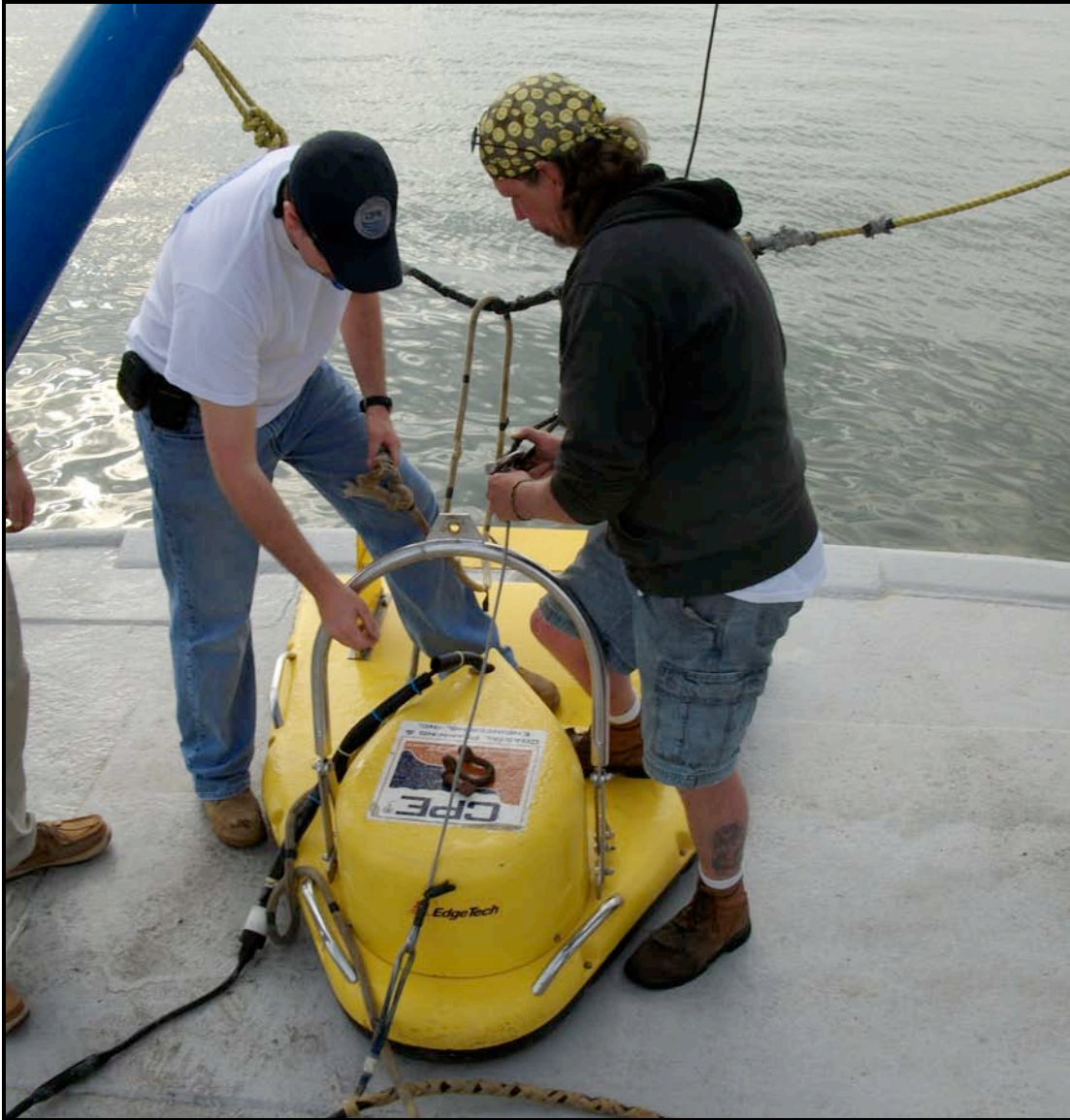
Figure 17. Launching the EdgeTech 512i Sub-bottom profiler.
