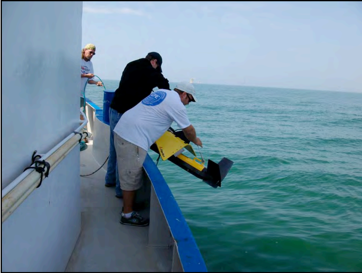
Figure 16. Launching the EdgeTech 4200-HFL side scan sonar.
