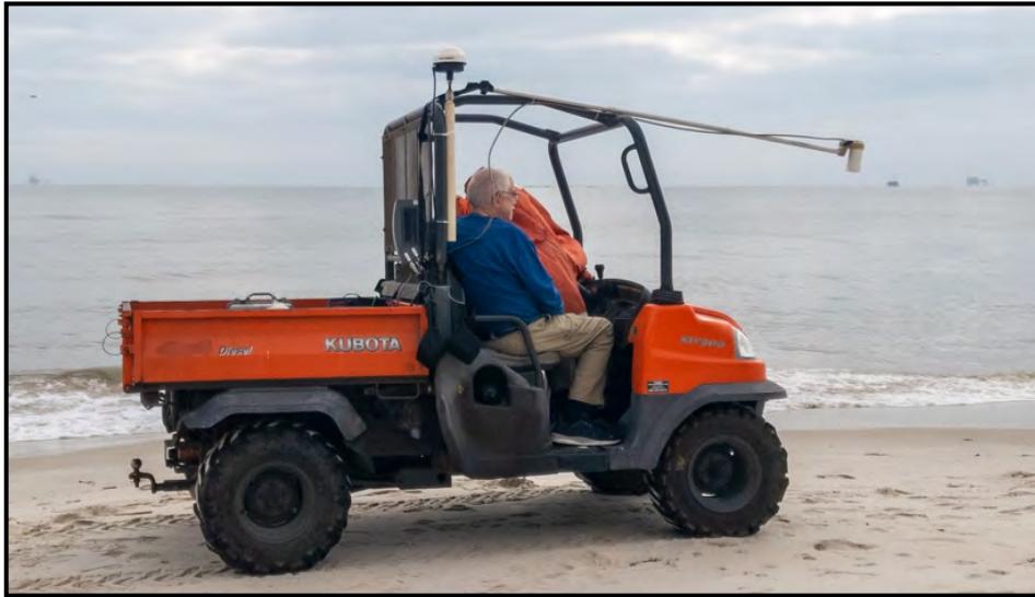
Figure 5. Kubota with mounted Hemisphere DGPS and G-858 magnetometer.
