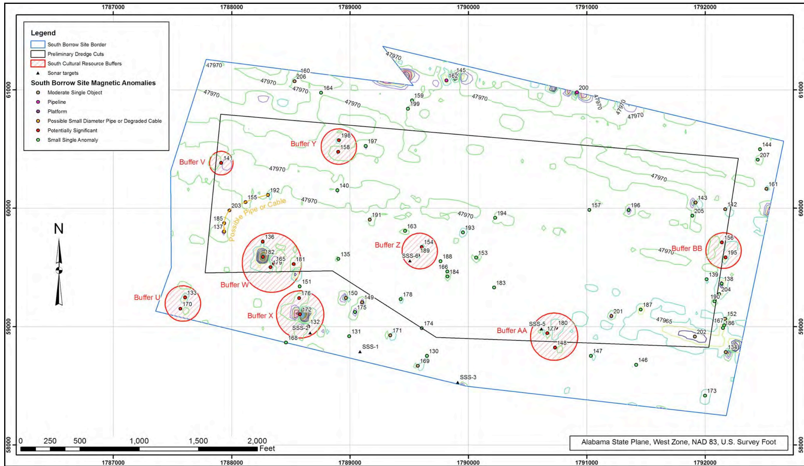
Figure 43. Magnetic contour map of the South Borrow Site investigation area with anomalies.
