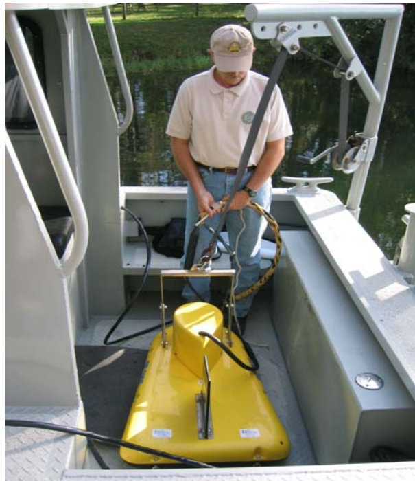
Figure 8.– Edge Tech SB216 full-spectrum “chirp” towfish.
