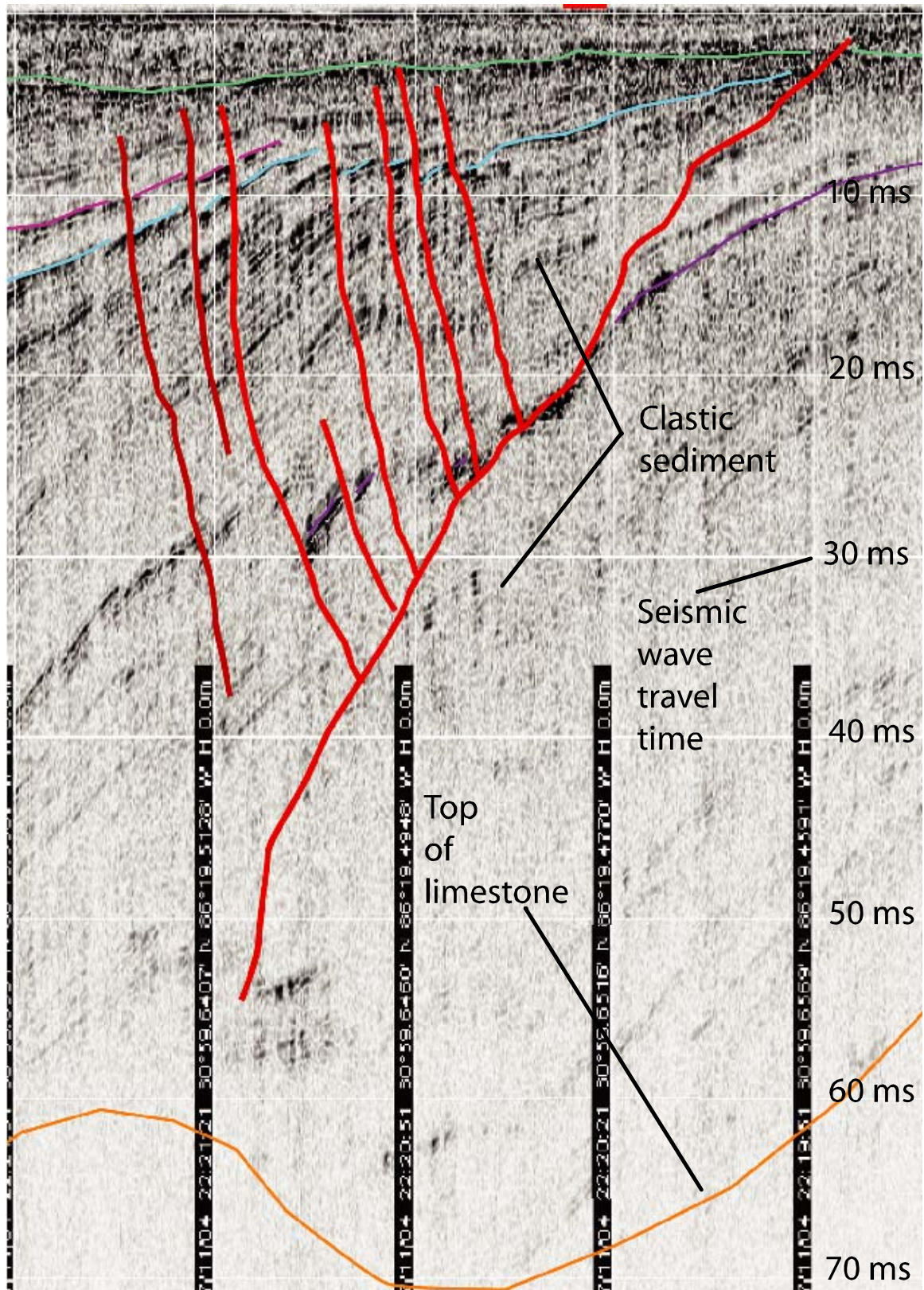
Figure 10.— Interpretation of seismic data from near the center of Lake Jackson.
